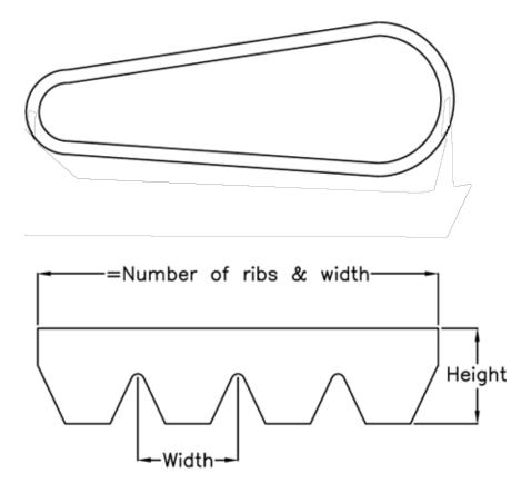
$\begin{array}{ll} \text{Datum Llength} = 1130 \\ \text{Height} &= 3.5 \\ \text{Number of ribs} = 5 \\ \text{Pitch} &= 2.34 \end{array}$
